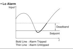
■ ON DELAY TIME: The relay status does not change until after the preset ON Delay Time (TD) once the signal input goes across the threshold.
