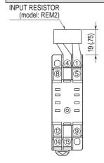
Input shunt resistor attached for current input.
