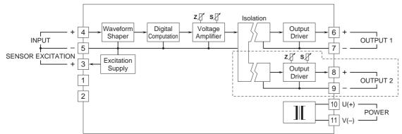
Remark 1: The section enclosed by broken line is only with 2nd output option.
