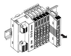
• Removing an intermediate module
