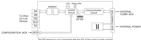
The FG terminal is not connected with the FG of the power supply module.
