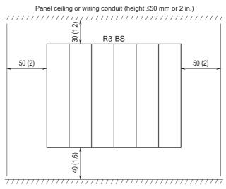
Panel bottom or wiring conduit (height ≤50 mm or 2 in.)
