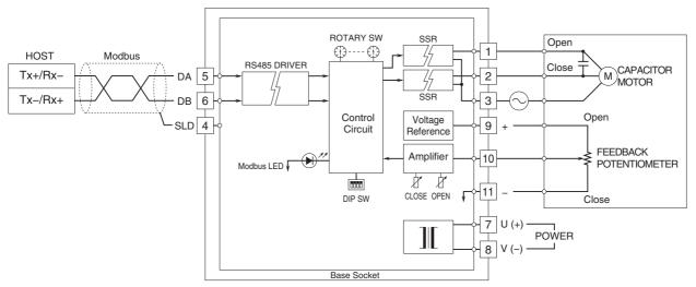
Note: Notice that making motor wiring with limit switch, every time the switch operates, can be causing stress on SSR.
