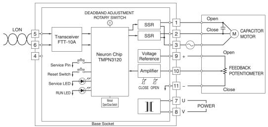
Note: Note that when limit switches inserted in motor wiring, the making/breaking may cause stress on the SSRs.
