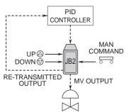
• Control loop utilizing pulse duration output from a computer
