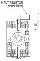
Input shunt resistor attached for current input.
