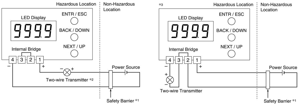
\*1. A safety barrier must be installed for the intrinsic safety.
