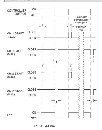
N.O. or N.C. selectable with jumpers. (a or b of CH1 START, CH1 STOP, CH2 START or CH2 STOP)
