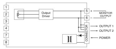
Note: Output 1, 2 and monitor outputs are all internally connected.
