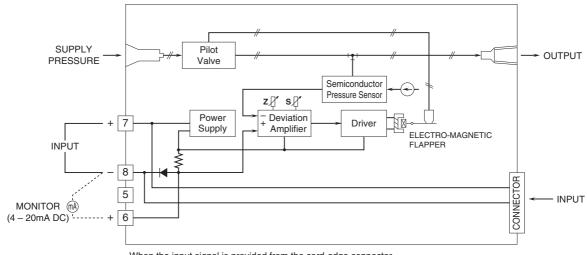
When the input signal is provided from the card-edge connector, the front terminals are not available for use.
