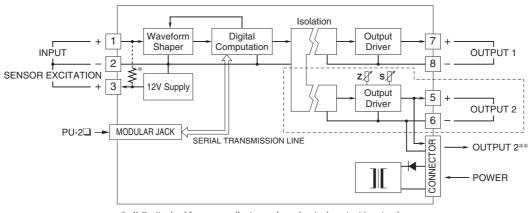
\* 4kΩ attached for open collector and mechanical contact input only. \*\*1 output type has the output 1 connected to the card-edge connector in parallel. Remark 1) The section enclosed by broken line is only for 2nd output channel.
