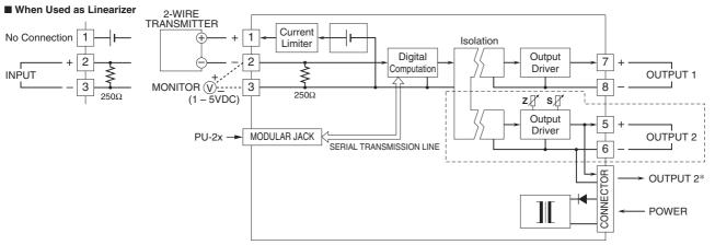
\*1 output type has the output 1 connected to the card-edge connector in parallel. Remark 1) The section enclosed by broken line is only for 2nd output channel.
