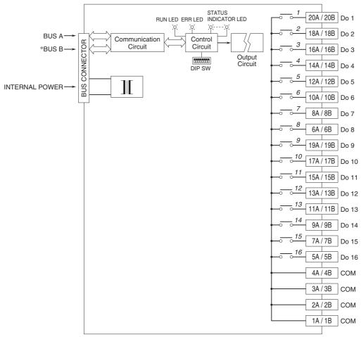
Numbers in italic indicate LED No.s assigned to the front panel LEDs.
