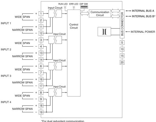
\*For dual redundant communication. NOTE: Connect either wide or narrow span terminals for each channel.
