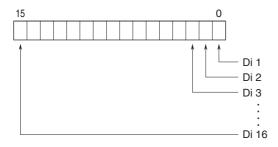
Note. Di 9 – 16 data is not practical discrete input data. It is "output completion status" internal data.
