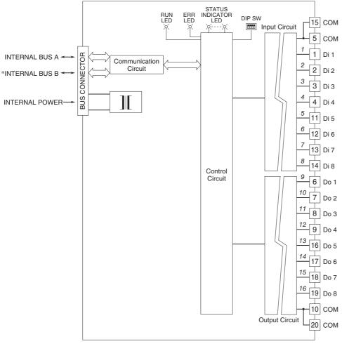
Numbers in italic indicate LED No.s assigned to the front panel LEDs. \*For dual redundant communication.
