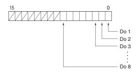
Note. For 4-bit length ON/OFF control mode, Do 5 through Do 8 are unavailable.
