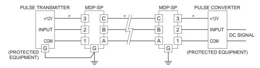
\*When there is no need of power supply, the cable is also unnecessary.
