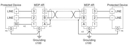
\*1. Leave Terminal A when the shielded twisted-pair cable is not provided.
