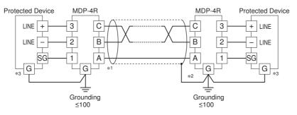
\*1. Provide electrical insulation with insulating tape and the like so that the live part is not exposed, as over voltage may generate on the shield wire.
