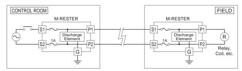
The M-RESTER must be connected with its terminals S1 and S2 faced on power source side in order that the fuses would be blown in case of shortcircuit of the discharge element.
