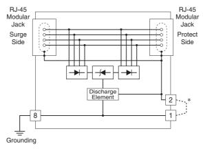
\*Remove the shortcircuit bar when the LAN cable's shield wire is floating.
