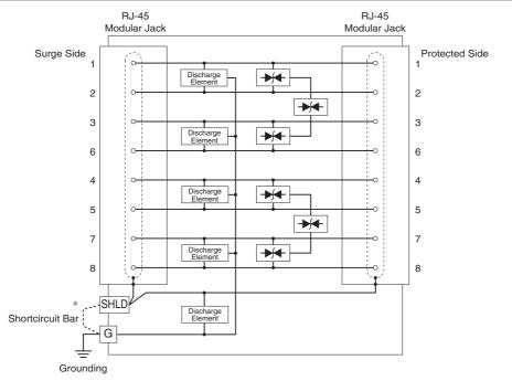
\*Remove the shortcircuit bar to make the LAN cable's shield wire floating.
