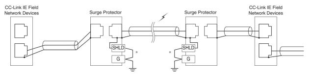
\*LAN cable's shield wire (SHLD) is 'earthed' when shortcircuit bar is connected. Make sure to connect the shortcircuit bar when you use shielded LAN cable.
