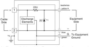
\*1. The zenor diode has polarity. Zero-cross signal cannot be connected.\*2. Use only when the signal line require functional grounding. This is NOT for surge protection.
