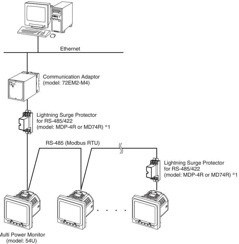
\*1. Insert lightning surge protectors recommended in this example if necessary.
