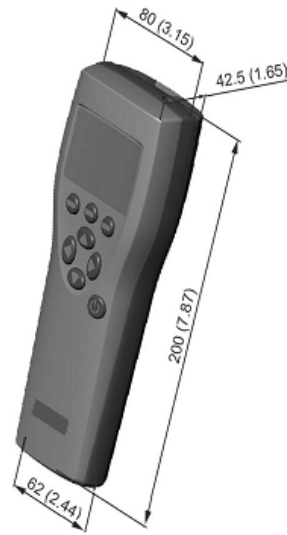
MI70 indicator dimensions in millimeters (inches)
