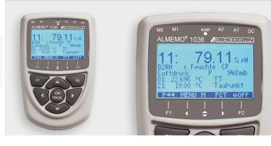
Reference measuring instruments for humidity and temperature **High-precision measurement** with the Pt100 psychrometer and Pt100 sensors **Resolution Temperature 0.001 K** Relative humidity 0.01 % Dew point 0.01 K
