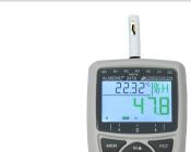
Professional measuring instrument, 1 measuring input, Data logger with integrated memory, Integrated sensor for temperature, atmospheric humidity, atmospheric pressure
