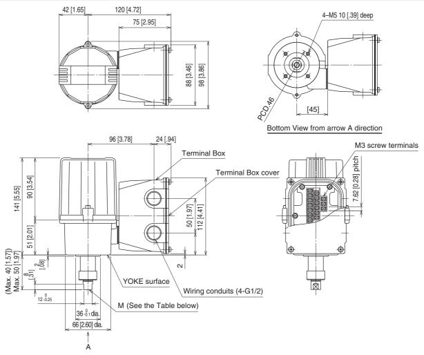
The dimension in ( ) is when the stroke is set to 5 to 10 mm.
