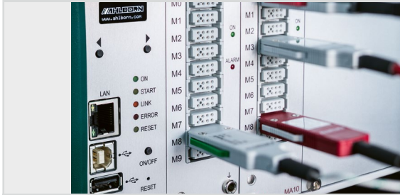
Ports for ALMEMO® sensors and for networking (OLED status display)
